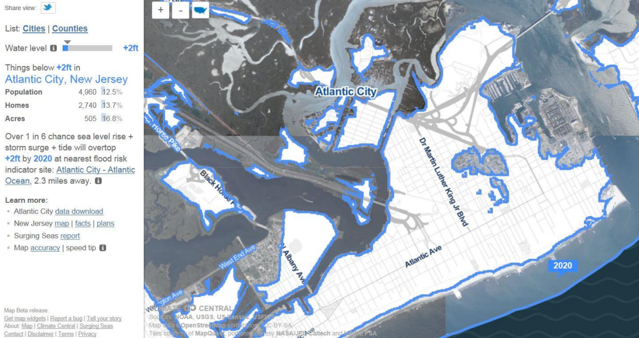
Figure 1: Map of Atlantic City from www.climatecentral.org showing the impact of a 2 foot rise on storm surge when combined with a high tide such as occurred during Superstorm Sandy.
